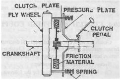
Fig. 2 Single plate clutch
