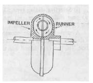
Fig 3 Fluid coupling
