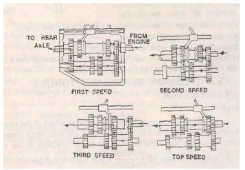
Fig 5 Sliding type gearbox for 4 speeds
