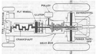
Fig 1 Power Transmission system of Tractor
