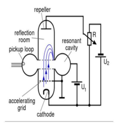
The reflex klystron (also known as a Sutton tube after one of its inventors, Robert Sutton) was a low power klystron tube with a single cavity, which functioned as an oscillator. It was used as a local oscillator in some radar receivers and a modulator in microwave transmitters the 1950s and 60s, but is now obsolete, replaced by semiconductor microwave devices.
